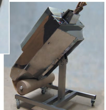
The machine tilts up to an angle of 45 degrees in its frame to alter the height at which cushions are dispensed.
