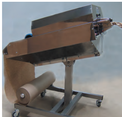
The machine tilts up to an angle of 45 degrees in its frame to alter the height at which cushions are dispensed.
