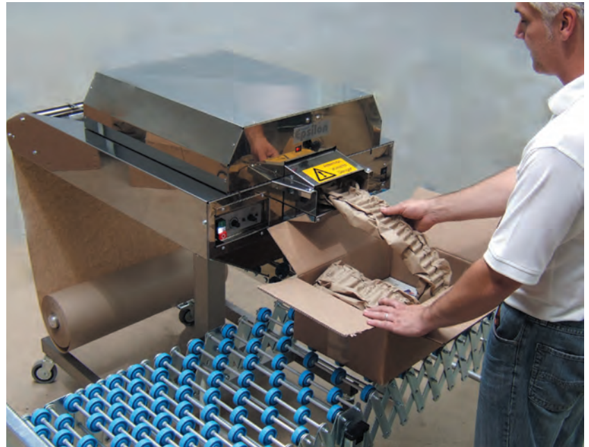
Epsilon produces bulky void fill straight into the box
